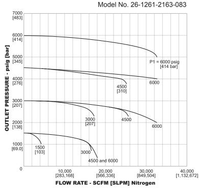
The curves above were generated using analytical methods - error is estimated at  $\pm 10\%$
