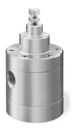
TESCOM 26-2900 Series is a dome loaded, negative bias, backpressure tracking regulator with a balanced main valve. This regulator controls upstream pressures up to 1000 psig / 69.0 bar with spring bias setting.
