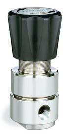
TESCOM 44-2300 Series is a compact, lightweight, single-stage backpressure regulator for specialty, flammable, and industrial gas flows of less than 4 SCFM / 113 SLPM. Diffusion-resistant metal diaphragm seal ensures gas purity and integrity.
