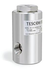
TESCOM 44-4200 Series is a high pressure, dome loaded, pressure reducing regulator with a  $C_V$  = 0.80 or 2.0 available. This regulator is rated up to 6000 psig / 414 bar inlet and 5000 psig / 345 bar outlet.
