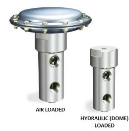
TESCOM 54-2800 Series high pressure, high flow, pressure reducing regulator is designed for hydraulic applications. Inlet and outlet rated up to 5000 psig / 345 bar;  $C_V = 8.0$  for high flows. Air operated and dome loaded versions are available. Hardened Stainless Steel seat and poppet for excellent wear resistance.
