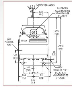
(standard for pressure range 3SS, 80SS or 150SS) 10 amps @ 125/250/480 VAC; 2 amps @ 600 VAC;
