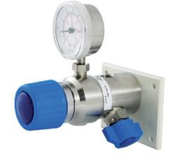
TESCOM Ultra High Purity MiniLabo 2 is a point-of-use regulator for high purity applications with a compact, modular ergonomic design. All connections are 1/4" Internal VCR<sup>®</sup> for reduced leak rates.
