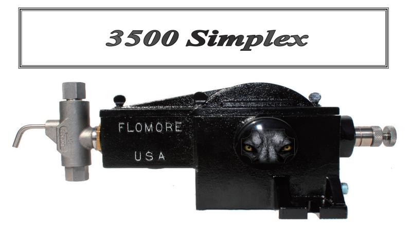
\*The Flomore 3500 series chemical injection pumps are electric driven, positive displacement pumps utilizing C-faced motors and common gear reducers. The gear reducers are available in 15, 30, 60, and 120 strokes per minute configurations. By utilizing even further flexibility of a wide variety of plunger sizes, the 3500 Series can fill many application requirements of different flow and pressures.
