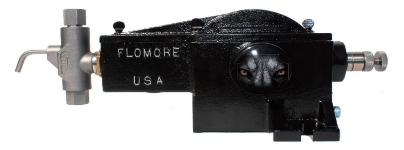
\*The Flomore 3500 series chemical injection pumps are electric driven, positive displacement pumps utilizing C-faced motors and common gear reducers. The gear reducers are available in 15, 30, 60, and 120 strokes per minute configurations. By utilizing even further flexibility of a wide variety of plunger sizes, the 3500 Series can fill many application requirements of different flow and pressures.
