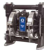
Husky 307 3/8 in (9.4 mm) connection Max flow: 26 lpm (7 gpm) Polypropylene, acetal
