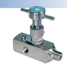
Century Valve CM40 and CM40DB gauge root valves are design for numerous piping and instrument applications. With connections ranging from flanged, butt weld, socketweld, and threaded they are suitable for most process and piping connections. All root valves are equipped with 3/8" roddable bore, in line replacable seat, and Century's patented non-rotating, firesafe bonnet assemblies. Meets ANSI B31.1 and B31.3 codes.
