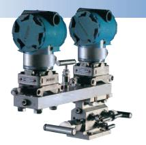
Century Valve's Direct Mount system is designed for the installation of instruments on fiscal metering applications. The system provides close coupling to the orifice tap and full porting to reduce any possible measurement inaccuracy through induced square root error. The system also has a range of other components to ensure the complete installation has full porting and the flexibility for single or multiple mounting of instruments.
